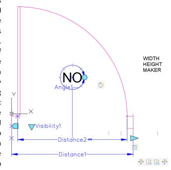
item 9.4. In the properties of external linear parameter set the NUMBER OF GRIPS to 1 and set DIST TYPE to LIST and add distance values of 80, 90, 120. Define parameter VISIBILITY and add 2 visibility states L and R. Then, make appropriate lines invisible for these states. Using BTESTBLOCK command test the dynamic block. Save the block to drawing file named DOOR BLOCK.DWG.
