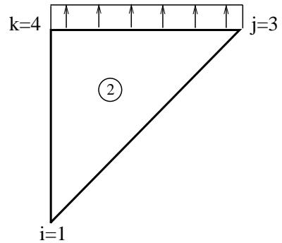
$$\mathbf{f}_b^{(2)} = \underbrace{- \int_{\Gamma_{13}} \mathbf{N}^{(2)T} q_n d\Gamma}_{redukcja} - \int_{\Gamma_{34}} \mathbf{N}^{(2)T} q_n d\Gamma - \underbrace{\int_{\Gamma_{41}} \mathbf{N}^{(2)T} q_n d\Gamma}_{w.b. q_n=0}$$
