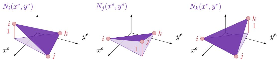
$$\mathbf{N}^e(x, y) = [N_i^e(x, y), N_j^e(x, y), N_k^e(x, y)]$$
